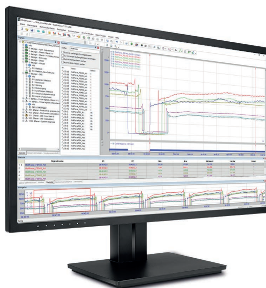
All sub-windows like signal tree, signal strips, value tables, search dialog etc. can be positioned freely. Markers can be used to measure signal characteristics quickly and easily.
