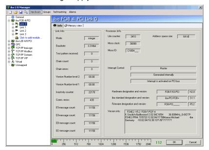
You get further information about the connected devices when you click on the device module in the tree. In the right part of the dialog you will then get general information (see above) but also the signal tables for analog and digital signals beneath the corresponding tab. Moreover, the actual values are displayed in the tables.
