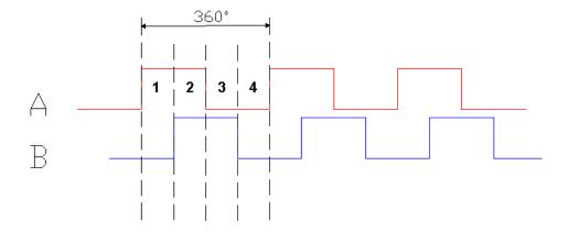
To be able to use the input channels A and B within an up/down counter, there needs to be decided when the counter will count up or count down.
