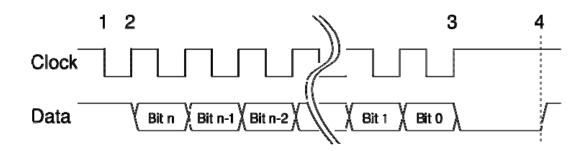
After the data has been read from the serial data line, the ibaPACO-4 device converts the binary or gray value towards a 28 bits signal. If the encoder uses a parity bit, the ibaPACO-4 device will remove the parity bit from the serial data.
