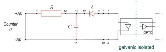
By default the counter input is suited for pulses with a nominal voltage of 24 V.
