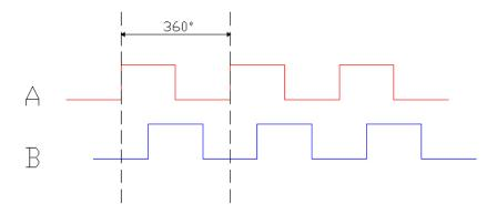
The edge separation for an optical quadrature encoder between any two adjacent edges is ideally 90 electrical degrees. Since there are four 90 degree periods in a standard 360 electrical degree cycle, this amount of separation is referred to as being in quadrature.
