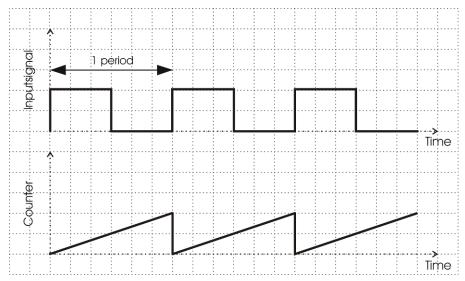
In order to make the measurement more accurate, the integration time can be extended over several periods. This can be done by changing the integration factor, so the calculation update is initiated every 2<sup>nd</sup>, 4<sup>th</sup>, 8<sup>th</sup> or 16<sup>th</sup> rising edge. More information on how to set up the integration factor is provided in chapter 8.8.2.
