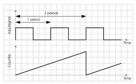
ibaPDA gets always a counter value which is normalized to an integration factor of 16. So the counter value needs to be adapted by the ibaPACO-4 device to correspond with 16 periods of the input signal.
