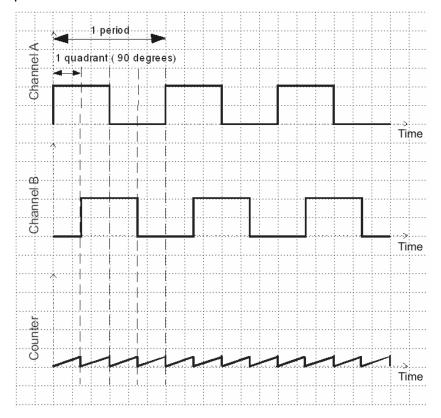
In order to make the measurement more accurate, the integration time can be extended over several quadrants of a period. This can be done by changing the integration factor, so the calculation update is initiated every 1<sup>st</sup>, 2<sup>nd</sup>, 4<sup>th</sup> or 8<sup>th</sup> rising period. More information on how to set up the integration factor is provided in chapter 8.8.2.
