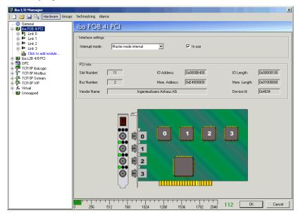
On the next tree level the view provides an overview about the communication parameters of all FO-links. A permanent change in Baudrate indicates that no telegram is received. This is either due to a missing or faulty fiber optic cable connection or to the fact that the voltage supply is not available for the device connected to the board.
