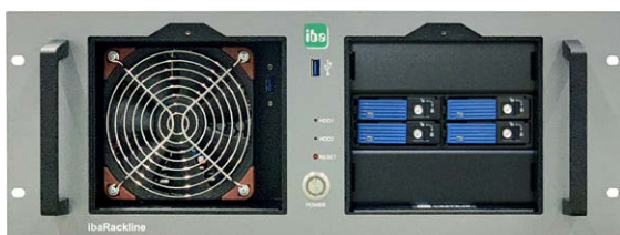
Front view ibaRackline without cover panels
