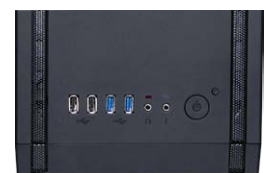
Interfaces on the housing top of ibaDeskline
